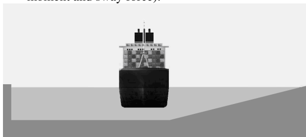
Figure 2 Cross section of a container carrier sailing with her side above the start of the slope
